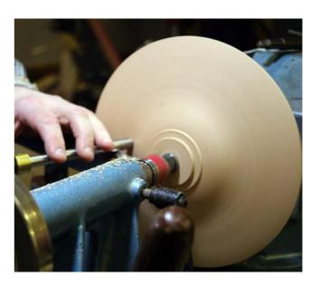
possible from his gouge Pat than used a rounded negative rake scraper to achieve a glass like surface which he then sanded to 400 grit. He also demonstrated the technique using a round skew chisel that was very effective.
