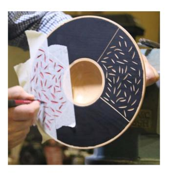
He used a point of a skew to mark the making tape 1/4" back from the edge front and back and from the edge of the bowl. A point tool was used to mark into the surface of the platter.
