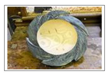
An Ash bowl blank was mounted on a faceplate and trued up on the lathe working from the centre of the blank towards the rim, so, cutting with the grain to prevent tear-out. A spigot was prepared for mounting the blank in a chuck later and the centre was marked for relocating on a jam chuck when the bowl was turned again after hollowing. The outside of the blank was then shaped to get a pleasing shape.
