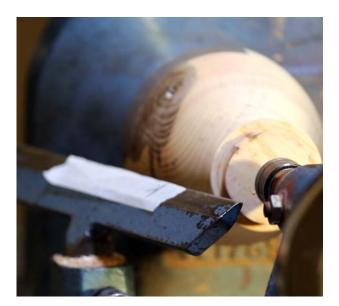
piece of packing between it and the bowl to prevent damage. He used the tail stock to centre the piece on the lathe. Seamus
