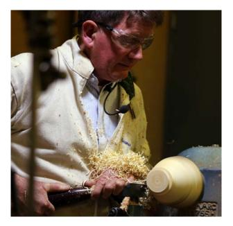
least 4 times when doing the outside and even more when doing the inside. Seamus mounted the shaped piece in the chuck and started on the outside. When he had the outside shape finalised he drilled the pith of the log out on both sides, using an
