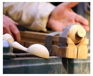
handle shape with a ball on the end. He then cut the turning in half lengthwise. He used a holding jig on the bandsaw that was a 90deg section with a slot cut on the bandsaw that enabled him to cut the round section of the spoon along it's length.
