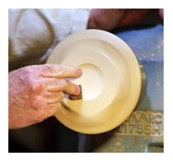
a jeweller so they could put some silver work in for sale. He used hot melt glue to centre a piece of 100mm x 5mm Ash onto a wooden back plate that was held to the lathe in a chuck. He faced off the wood and then made a shallow impression in the
