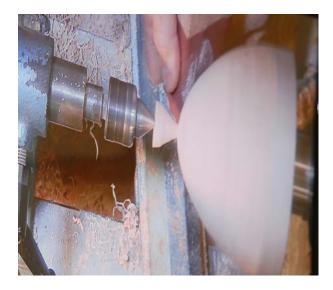
put a piece of masking tape onto the tool rest to mark the inside of the vessel. He then finished the outside of the piece. Being very careful when he was taking off the last piece. The piece was a conical shape.
