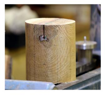
surface. He mounted the blank in a screw chuck and faced the end off. He used a bradawl to find the centre then he made a chucking point on that end. He also
