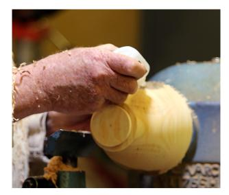
He finished the bowl to about 3 to 4mm and sanded with a pad. On the outside of
