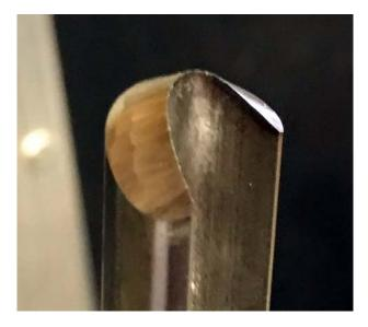
specially shaped by himself, one side has a long grind and the other a short grind. The angle on the top of the grind is very flat.
