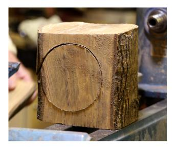
the blank from a log using a band saw, taking the blank from the centre of the log. This meant that the pith of the centre of the tree was still there. Seamus marked the position of the pith on each side up to the top surface and marked the line on the top
