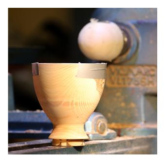
bowl to the hole he made when drilling out the pith. Explained that the wet wood was moving already to a different shape so before he reversed the piece to do the bottom he used a bit of gaffer type tape to support the edges of the cuts.
