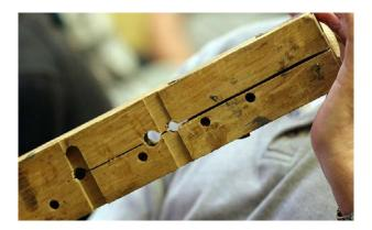
He used this preprepared turning for the rest of the demo. He had made a wooden faceplate that mounted in the lathe with a chuck. He had made a depression in the centre of the faceplate that let the back of the spoon go below the surface of the faceplate. He brought up the tailstock with nothing in it and used that to hold the spoon onto the faceplate. Using the tailstock in this way ensured the spoon
