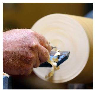
shaped the outside of the piece to a taper. When he had taken the shape as far as he could without making it too narrow behind the chucking point he mounted it in the chuck.
