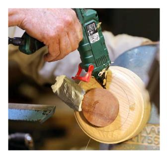
was absolutely square to the line of the lather bed. He then used hot melt glue to secure the spoon to the faceplate. He put some protective material around the handle so that it could be seen when turning was going on. He then removed the tailstock and took the centre out of the spoon. He finished with a sanding.
