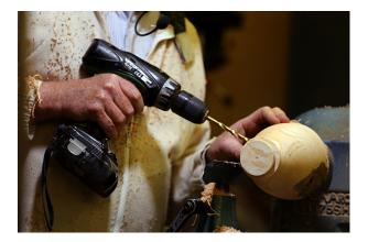
8mm bit. Super glue was used in the hole to stabilise the area around the pith. He
