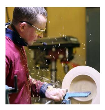
profile the lid to match the profile on the base. As before, he used a selection of gouges with differing profiles to try to achieve the best cut on this particular piece of Ash. Having satisfied himself with the finish the lid was sanded from P120 to P400 and the piece was removed from the lathe and reversed into a chuck to allow the inside to be cleaned out.
