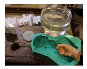
When using silicon rubber you need to be careful to avoid moisture while the mould is setting and Fast Cast Polyurethane will set in about 15 minutes so you will get results quite quickly. The type of material you use for the mould will depend on the desired result e.g. if you want to lift a lot of detail use a soft silicon mould material. It is advisable to use some sort of mould release to ease extraction of the cast. This could be wax, silicon or spray teflon.
