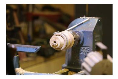
making cuts towards the headstock. When she got near to the pot she cut from the centre out and slightly undercut the pot. As before, she stopped frequently to assess the quality of the cut and decide how to proceed. When satisfied with the bottom Margaret cut two recesses or 'V's to disguise the lip of the bung where it was glued in. She then sanded the bottom and used the corner of the abrasive to clean the V-cuts.
