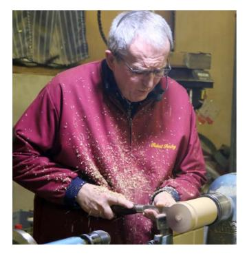
lead David used African Lead-wood, a dense, tropical, hardwood. After the blank was drilled it was mounted between centres and rounded to final diameter using calipers to assess progress. David reminded us to round over the ends of our calipers before sticking them onto spinning wood. Once the diameter was set the area for texture was marked out and the ferrule was fitted.
