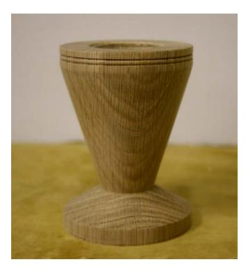
Now that the drilling was complete David set the shape of the candle using dividers to set, and record, measurements for the second candlestick he would make. He marked guidelines for the base and reduced the stem to about 40mm with a parting tool.
