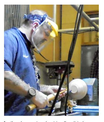
for the shear cut and not to allow it to become a scraping cut as we rounded the bowl exterior. Before removing the blank to turn it around Nick tidied up the base to prevent problems later when he would have problems accessing it.
