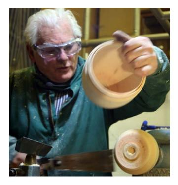
shoe before cutting it off the chuck. He used the piece of Ash left in the chuck to make a jam chuck. Reversed the form onto the jam
